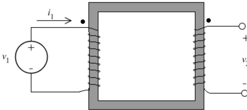
Figure 1: Two coils are magnetically coupled, wound around a magnetic core.
