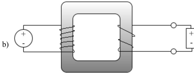
Figure 5: a) Step-up transformer, b) Step-down transformer
