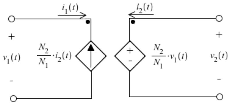
Figure 10: Ideal transformers represented through dependant voltage and current sources.
