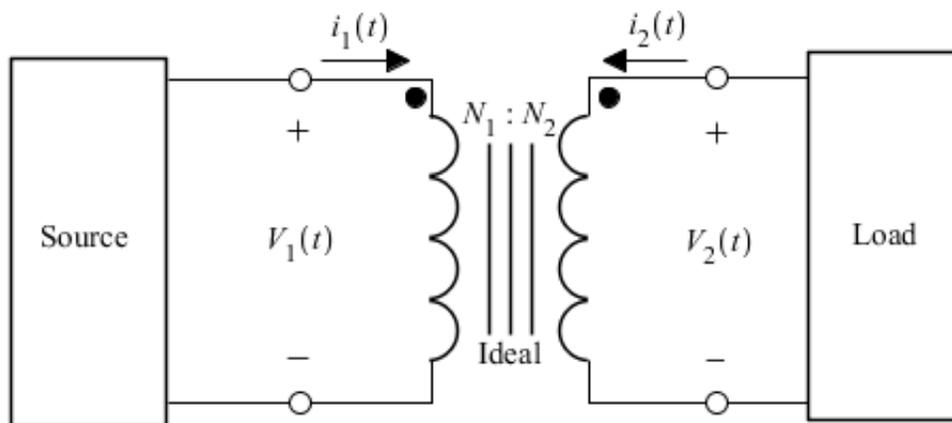
Figure 7: A source circuit and load circuit connected with an ideal transformer
