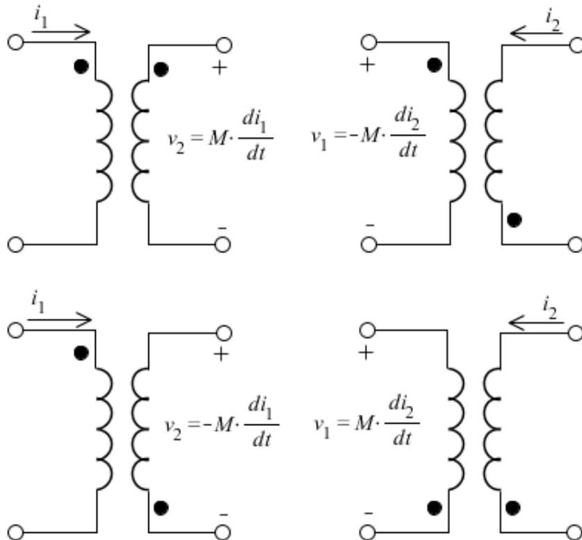
Figure 3: Induced voltage of coupled inductors.
