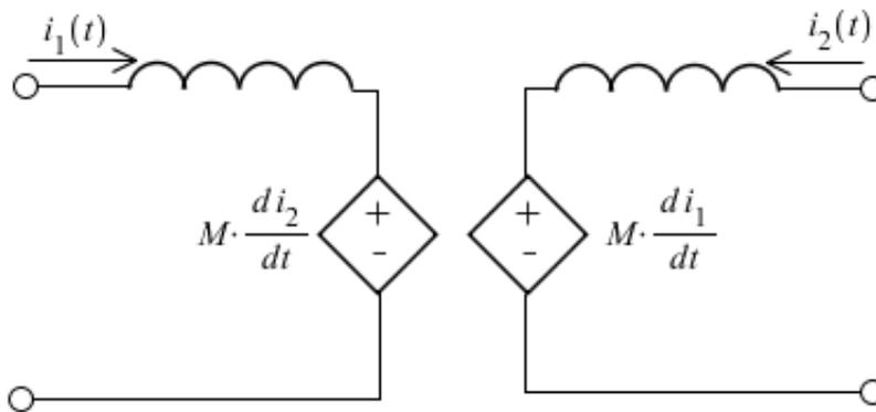
Figure 9: Inductors coupled via dependent voltage sources.
