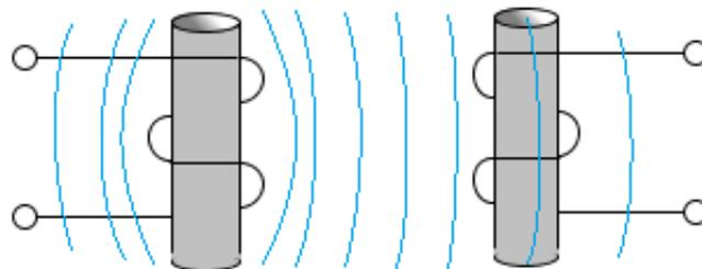
Figure 4: Flux lines cutting through the coils.
