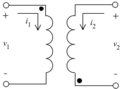
Figure 2: Coupled inductor with dot notation
