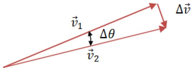
Fig. 3: Vector subtraction - small angle
