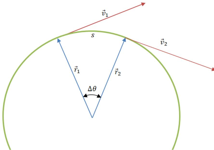
**Fig. 1: Particle in uniform circular motion**
