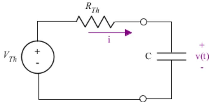
Figure 3: Capacitor and Thevenin circuit
