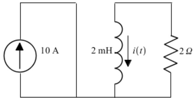
Figure 9: Circuit after  $t=0$  and before second switch
