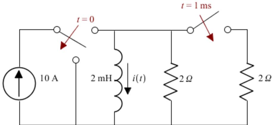
Figure 7: Inductor circuit with two state changes
