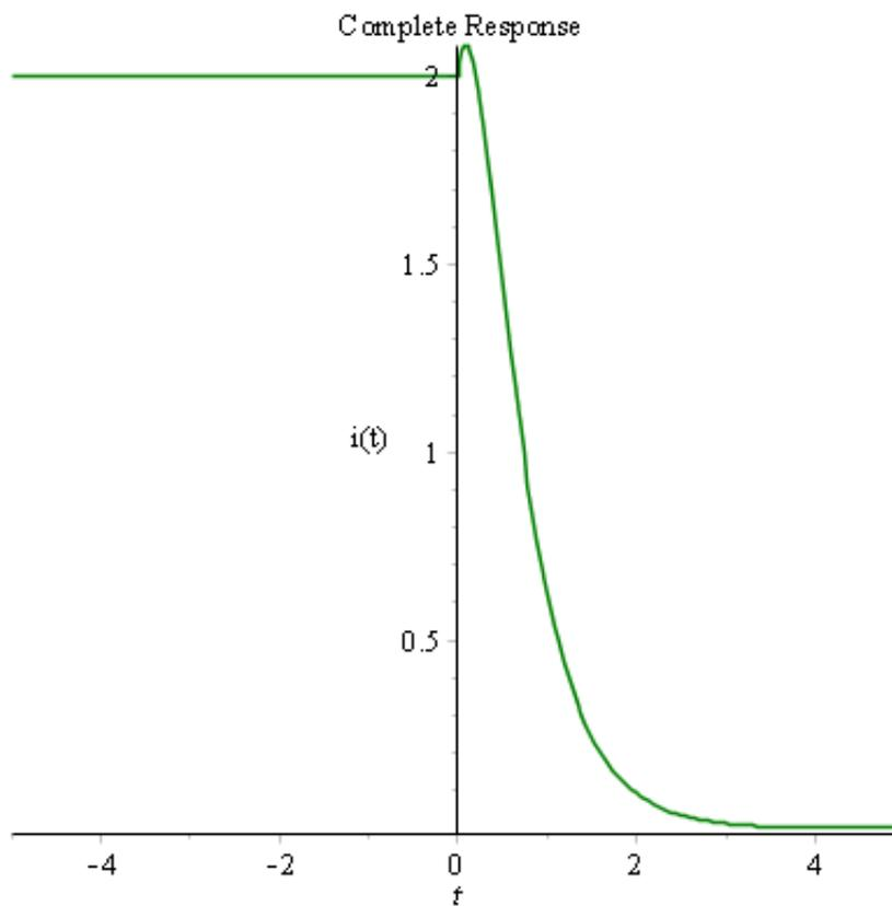
Figure 14: Complete response of LR circuit with exponential source.
