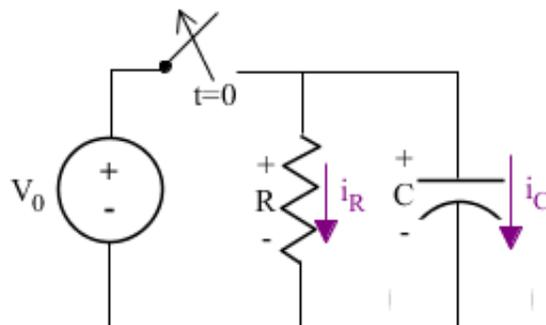
Figure 1: RC circuit
