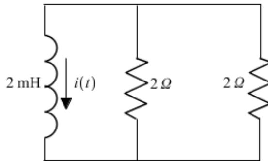
Figure 10: Circuit after  $t=1$  ms.
