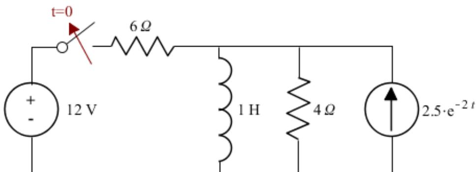
Figure 11: LR circuit with an exponential source
