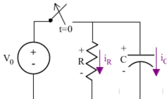
Figure 1: RC circuit with constant input
