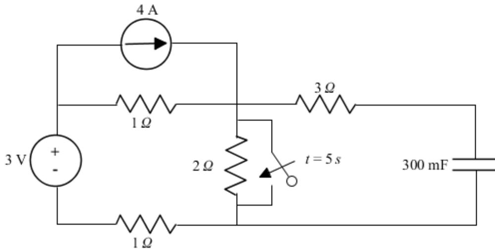
Figure 15: Constant sources with a capacitor
