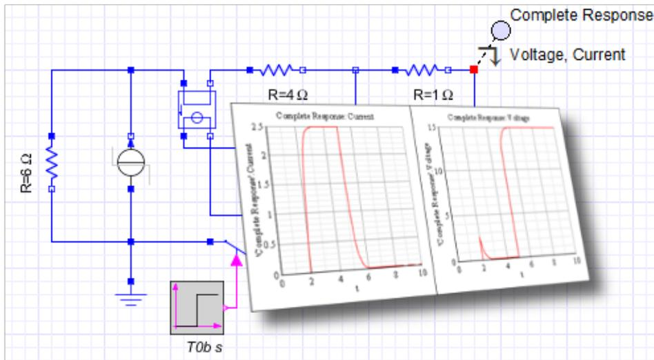
When non-linear elements such as inductors and capacitors are introduced into a circuit, the behaviour is not instantaneous as it would be with resistors. A change of state will disrupt the circuit and the non-linear elements require time to respond to the change. Some responses can cause jumps in the voltage and current which may be damaging to the circuit. Accounting for the transient response with circuit design can prevent circuits from acting in an undesirable fashion.
