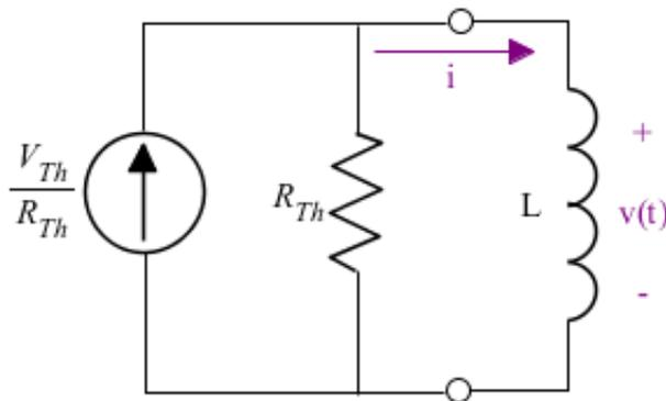
Figure 6: Inductor with Norton equivalent circuit
