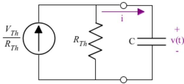
Figure 4: Capacitor with a Norton equivalent circuit
