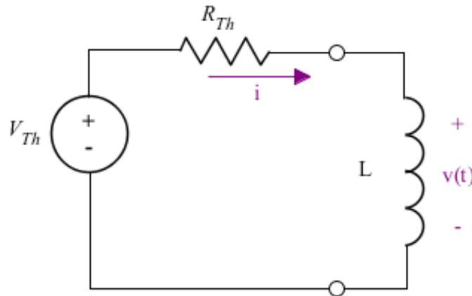
Figure 5: Inductor and Thévenin equivalent circuit
