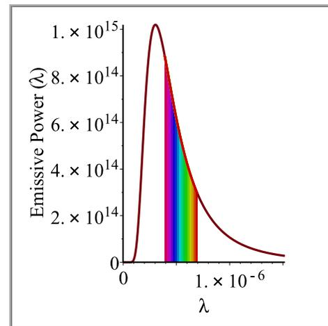
Figure 7: Emissive power vs wavelength chart with adjustable temperature.
