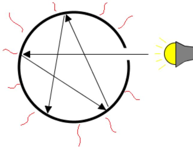
Figure 6: A black body as a cavity with a hole
