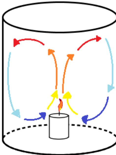
Figure 4: Natural convection. The hot air from the flame expands and rises above the denser cold air.
